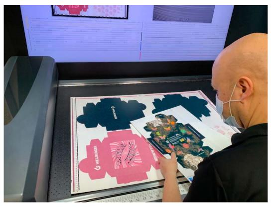
Bastian Pinsenschaum (Head of Technical Service, WEILBURGER Graphics GmbH) during the final  $\Delta E$  check of the flexo inks of the SENOFLEX® WB INKS FP DC series applied on the reverse side to the offset inks applied on the straight side. © Photo: STI Group, Meike Dihstelhoff
